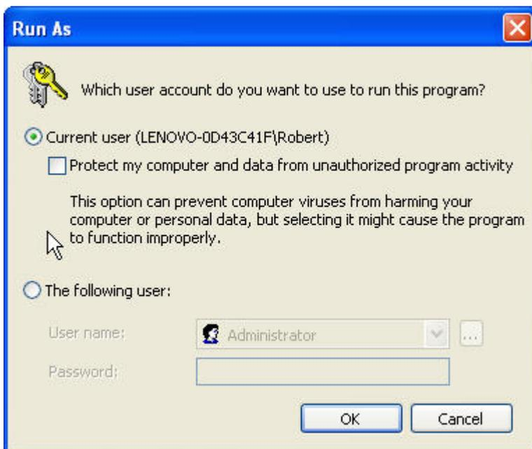
Figure 6 Deselect 'Protect ...' to run in Admin mode.
